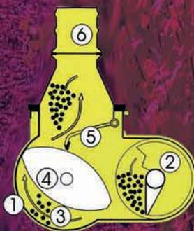
The monoblock unit (1) is manufactured in stainless steel AISI 304. The product comes from an auger (2), until inside of the pump (3), where the action of an elliptic rotor in stainless steel (4), through a separator valve (5), pushes it to the exit(6).
