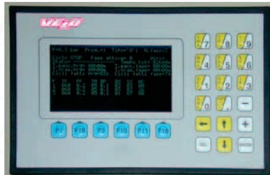
Quadro de controle - PLC
